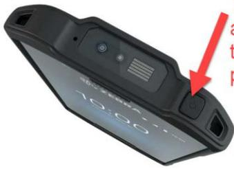
Turns the display on and off. Press and hold to reset the device or power off.
