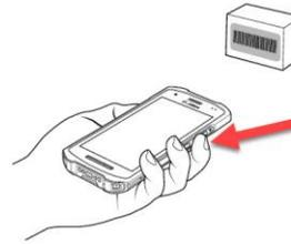
Press and hold the scan button. The red laser aiming pattern turns on to assist in aiming.
