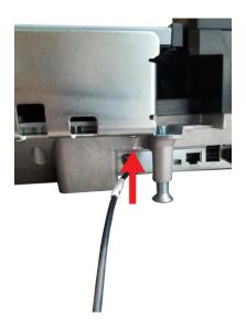
3. Grab the Power+ USB cable and plug into the rightmost port on right side of the scanner scale.
