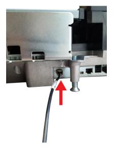
2. Grab the USB cable and plug it into the rightmost port on the right side of the scanner scale.
