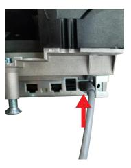
3. Assemble the Power Supply cables and plug it into the rightmost power plug on the right side of the scanner scale.
